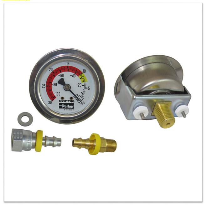
A vacuum gauge is used to check the condition of your fuel filters. Uses no power and will extend the life of your filters. Don't change the filters when dirt appears in the glass bowl but wait until the vacuum increases. Increased vacuum gives a warning that the filter is starting to get plugged up. Surprised many boats do not have this device on their fuel delivery system yet it costs less than \$100 installed.
