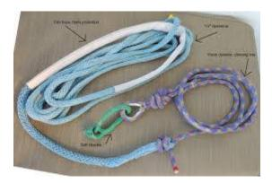
"With snubbers the objective is to get maximum stretch with minimum chafe. I have copied an idea from New England Ropes and created a line with very chafe resistant dyneema (blue line) from the deck cleat to just beyond the bow roller, and then with stretchy dynamic rock climbing line from the bow roller to the soft shackle. Above is a picture of version #1." Thanks to Evan for this new method.
