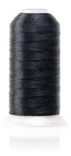
Goretex thread marketed under the name Tenera is very expensive (\$120 a spool) but so worth the price because it is UV resistant (also petroleum resistant to grease, etc.) Every bit of canvas should be made using Tenera. This thread will outlast the material. Use normal canvas thread and you will be restitching in 2-3 years. One summer in the brutally hot Sea of Cortez and you will have to restitch in 1 season. Comes in clear, white and black.
