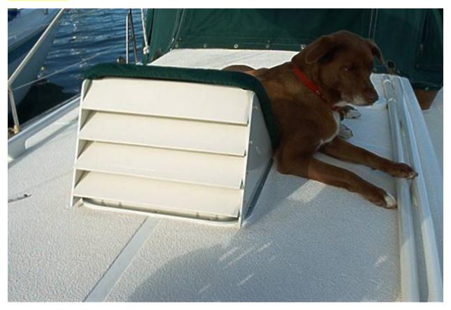
Keep the rain out and allow breeze to flow into the boat. Using a ½ sheet of 1/4" plywood I made these collapsible louvers based on my brother-in-law Buzz's design. They come apart and fold flat. Easy to put together allowing you to get maximum air flow when it's raining.
