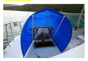
These units fit outside your hatch and increase the amount of air rammed below. They can be turned as needed. Slides into a small bag for storage.
