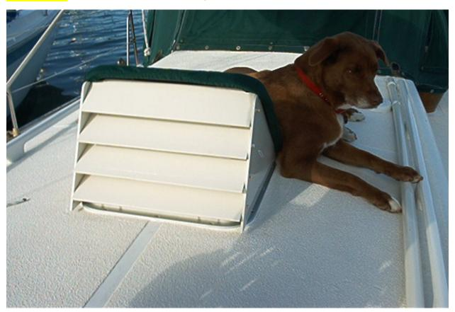
Keep the rain out and allow breeze to flow into the boat. Using a ½ sheet of 1/4" plywood I made these collapsible louvers based on my brother-in-law Buzz's design. They come apart and fold flat. Easy to put together allowing you to get maximum air flow when it's raining.
