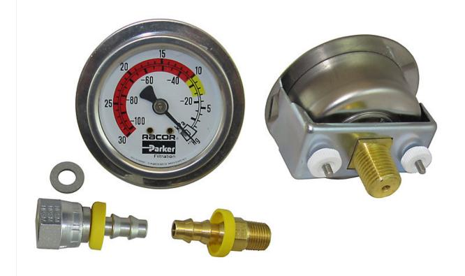
A vacuum gauge is used to check the condition of your fuel filters. Uses no power and will extend the life of your filters. Don't change the filters when dirt appears in the glass bowl but wait until the vacuum increases. Increased vacuum gives a warning that the filter is starting to get plugged up. Surprised many boats do not have this device on their fuel delivery system yet it costs less than \$100 installed.
